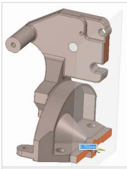
**Geometric Inferencing** works unobtrusively and in real time to highlight design similarities, such as equal radius holes or coplanar surfaces, during geometry creation and modification, improving user productivity.
